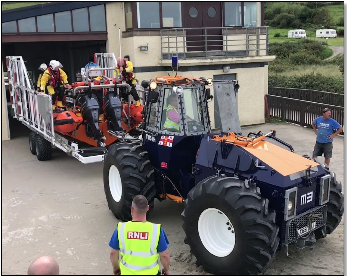
RNLI Amphibious Tractor Made in Knighton for Lifeboat Transfer
